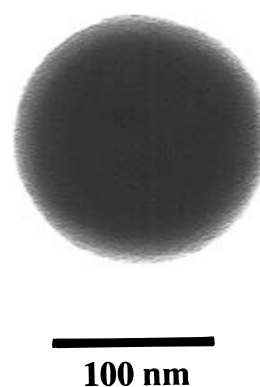
Figure 9. TEM micrograph of a silica particle coated with 1077-1158 in THF/CP with f_{CP} = 0.82 . The TEM specimen was stained by \text{OsO}_4 .
